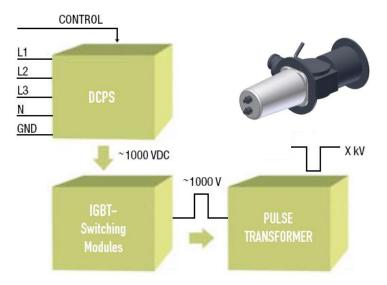
The DCPS is the main power source of the system. It converts the 3- phase line voltage to a regulated DC voltage. It charges up all the IGBT Switching Modules to a primary voltage around 1000V. An external trigger pulse enters the modulator, gating all the IGBT Modules and discharging some of the stored energy. The IGBT's are high-power solid-state switches, which can be turned on and off electronically, responding to the trigger pulse.
