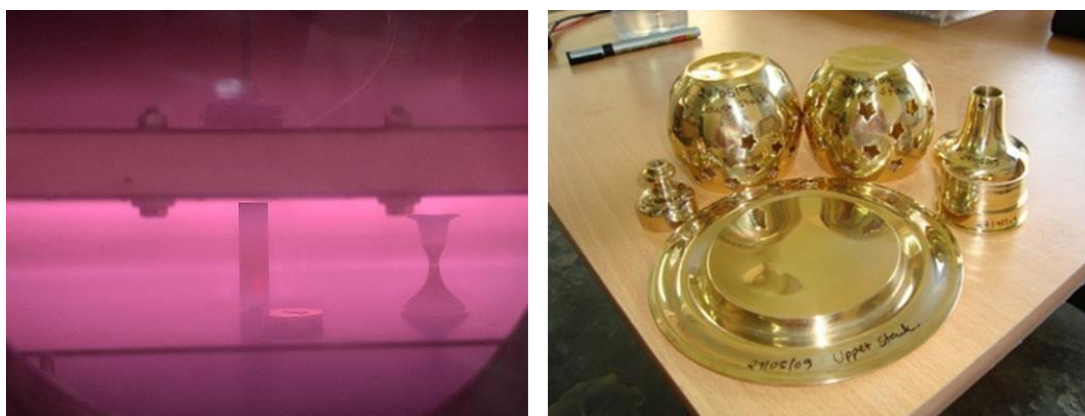
Figure 2: PECVD process to polymerize HMDSO and SiO x coated brass components.
